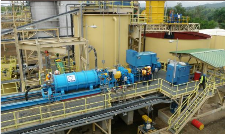
HyperSpargers™ oxygen addition
